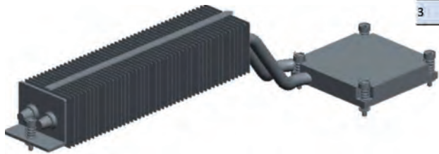
Figure 3. Detail of Heat Pipe Design for IC
