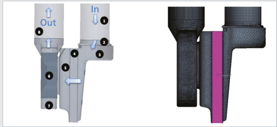
Figure 2: Detail of ducting geometry surrounding the evaporator and the corresponding computational mesh (evaporator is marked as component 4 in left image, and is highlighted in purple on right image).
